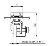
Cross terminal ø8mm for rebate up to 8mm according to EN62561-1.
